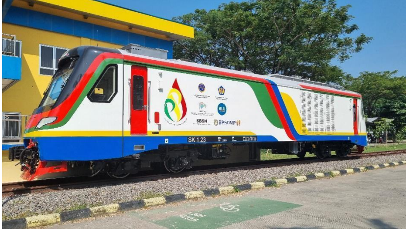
Track Motor Car (TMC) at PPI Madiun utilizing an electric motor system
