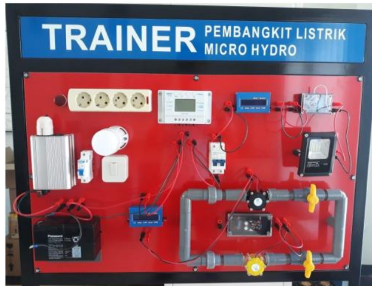
Figure 7. Generator prototype micro hydro
